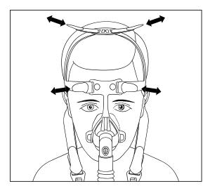
Adjust the upper headgear straps A1, A2, A5 and A6 to a comfortable tension.
